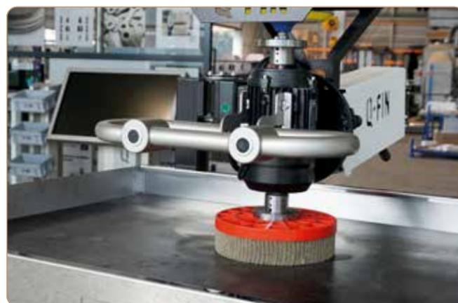
Edge rounding with the optional  $\varnothing 255$  mm disc brush.
